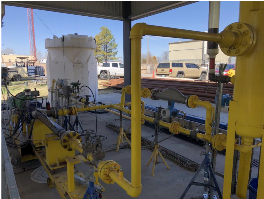
Figure 2.2 Photo of TUALP single-phase oil ESP flow loop
