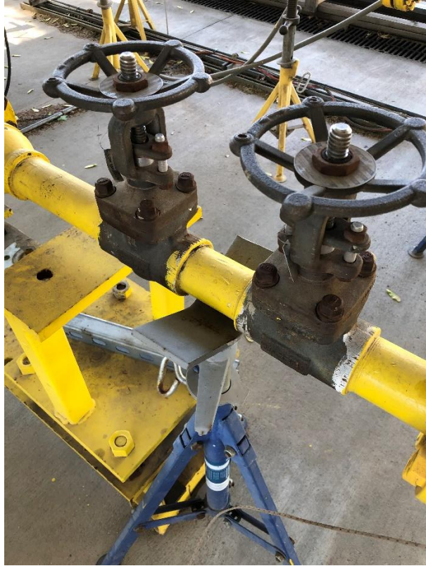
Figure A.1 Liquid flow control valve
