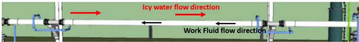
Figure A.11 Fluid Flow Schematic inside the Heat Exchanger
