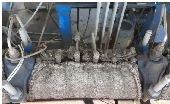
Figure 2.8 Top view of pressure measurement ports
