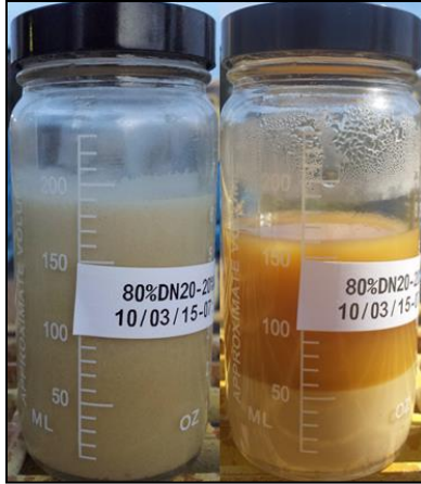
Figure 2.44 A sample 1 minute after collecting (left) and 1 day (right)
