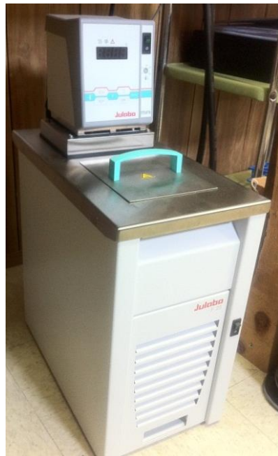
Figure A.10 Thermostatic bath and circulator for rotational viscometer
