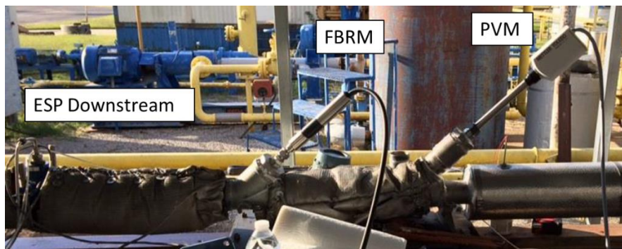
Figure 2.41 FBRM and PVM probe setup
