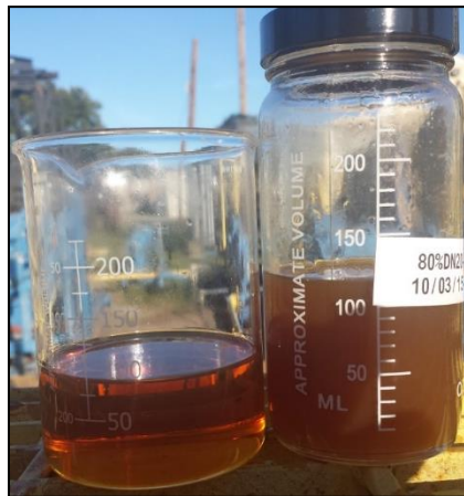
Figure 2.45 Pure oil (left) and remaining used oil after heating (right)
